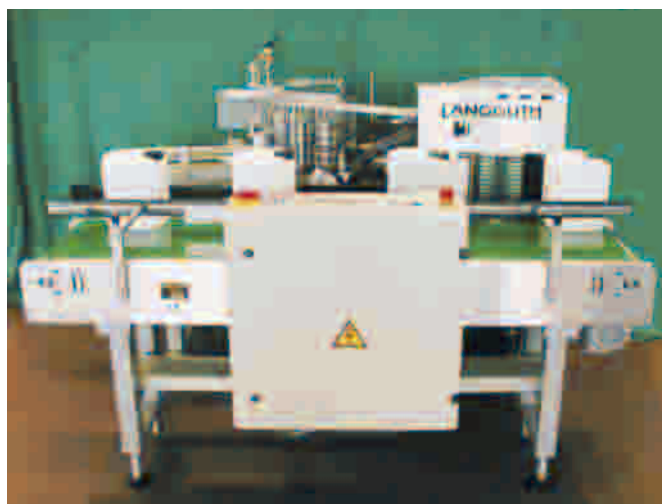
Photo shows the hot-melt labelling machine for large rectangular containers with patch label
